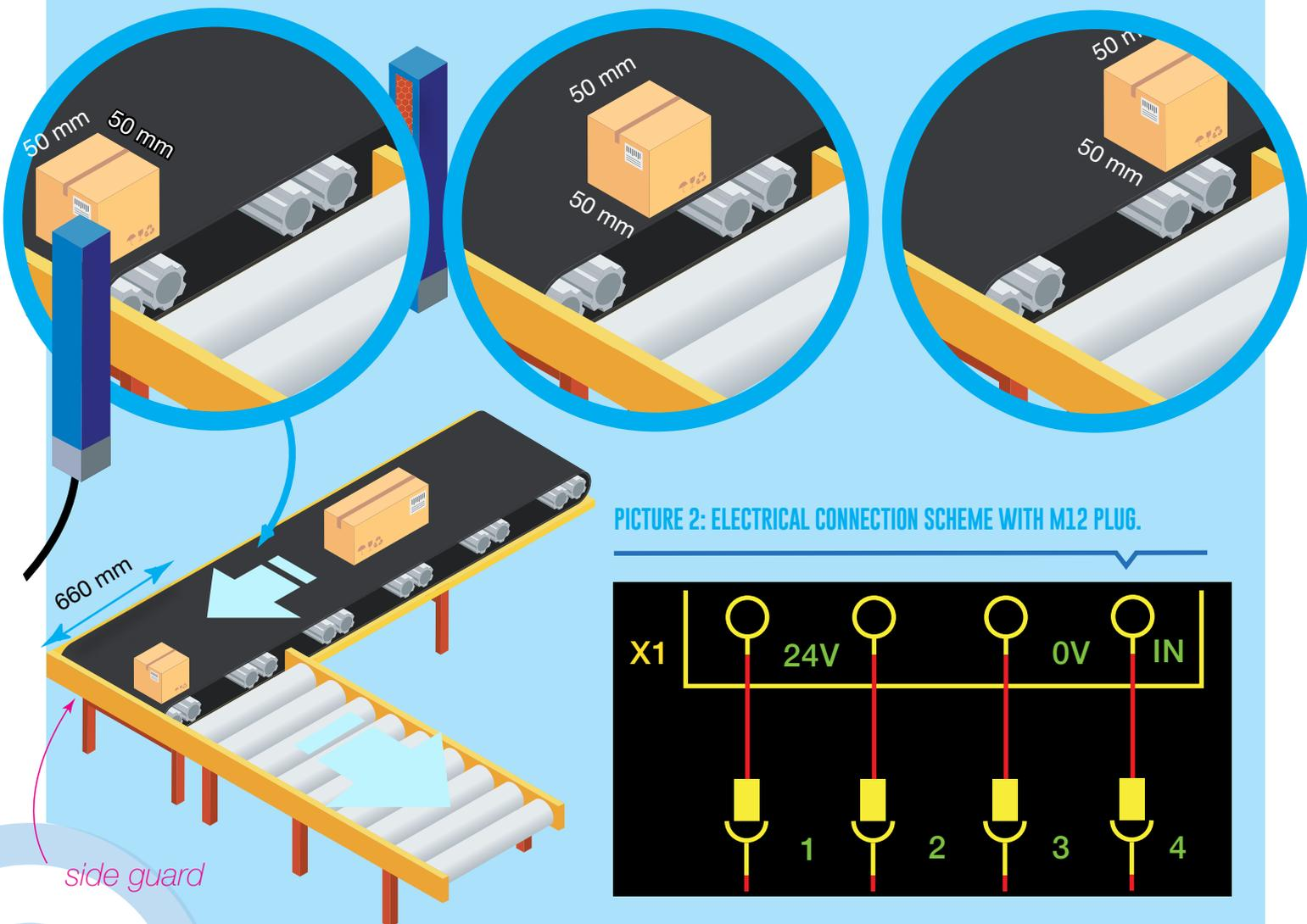
connector and do the Teach-in by pressing the single button on the sensor. The fact that the sensor is so easily configurable in turn allows the installation to be done even by less experienced operators.
